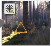
Set the crosshairs position: Point the probe at a distant object. Drag the crosshairs to the red laser dot. Warning: Laser!
