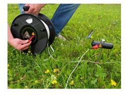
5. Use the Extension Cable to connect the Power Drum with the Power Electrode.
