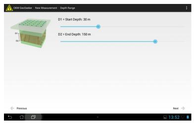
Figure 5.7: New Measurement - Depth settings
