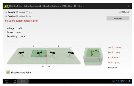
Figure 7.5: Instruction screen for setting up a measurement
