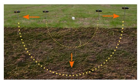
Figure 7.3: Power injection depth depends on electrodes distance
