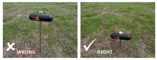
Figure 9.1: Electrodes need good electrical ground contact
