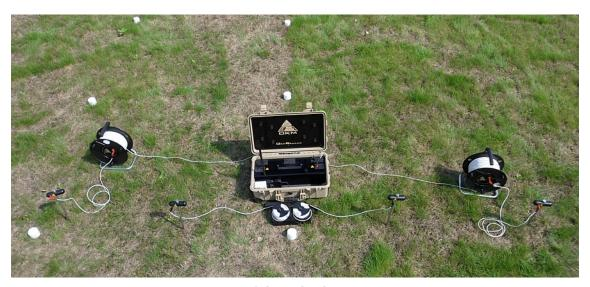
Figure 7.6: Arrangement of electrodes during Active Scan (Accurate)
