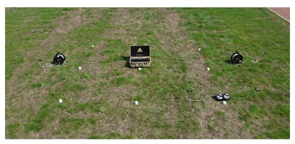
Figure 7.7: Arrangement of electrodes during Active Scan (Quick)
