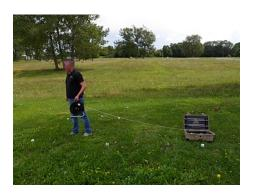
Unroll the cable of the Power Cable Drum by moving away from the Power Box until you reach the cable marker indicated by the Android application of your Tablet PC.
