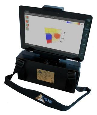
Figure 6.3: Tablet PC mounted to Controller
