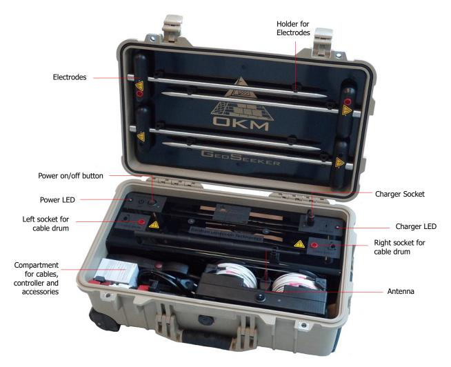
Figure 4.5: Control elements of the Power Box
