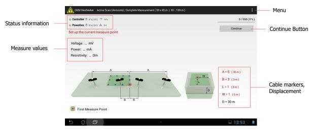
Figure 5.9: New Measurement - Arrangement of electrodes
