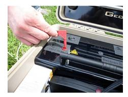
2. Connect the plug of the first Power Cable Drum into the appropriate socket of the Power Box.
