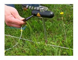
5. Connect the cable of the Voltage Cable Drum with the Voltage Electrode.
