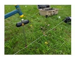
Put the Voltage Electrode next to the cable marker into the ground as deep as possible. Use a hammer if necessary.
