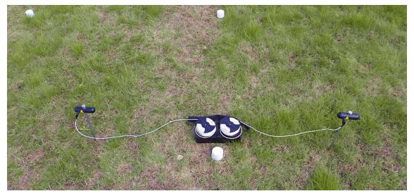
Figure 7.8: Arrangement of electrodes during Passive Scan
