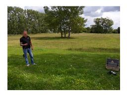
3. After reaching the end make a U-turn and bring back the cable to the cable marker indicated by the application of your Tablet PC. Unrolling the cable completely is necessary to get the right order of the cable markers and makes it easier to rearrange the electrodes afterwards.
