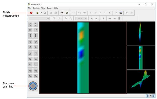
Figure 7.10: Graphical representation of Ground Scan
