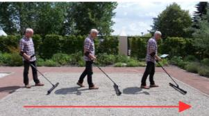
Figure 7.11: Ground Scan in vertical and horizontal mode
