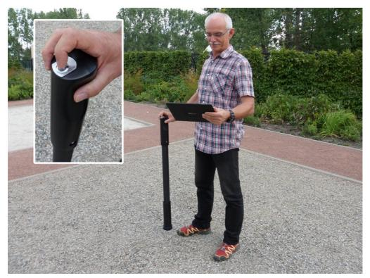
Figure 6.1: Using the detector in vertical mode
