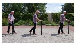
Figure 7.5: Probe should always point downwards and should not be turned
