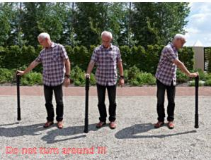
Figure 7.6: Pivoting or turning of the probe falsifies the measurement
