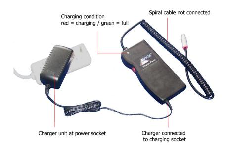
During the charging process of the Power Pack, the LED is shining red continuously. As soon as the LED shines green, the Power Pack is charged completely and must be disconnected from the charger.
